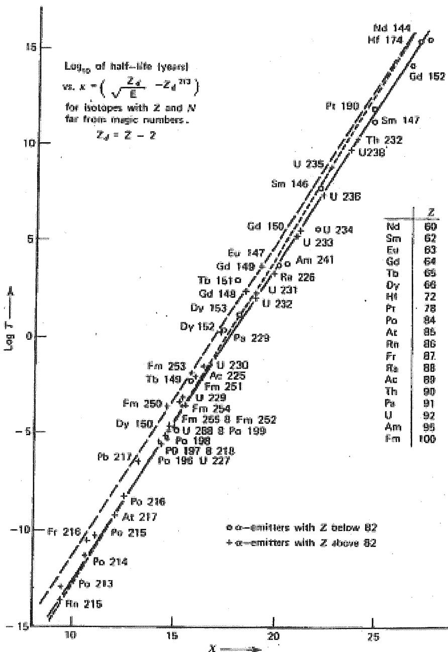
Figure 5-9. Plot of  $\log_{10} 1/\tau$  versus  $C_2 - C_1 Z_d / \sqrt{E}$  with  $C_1 = 1.61$  and a slowly varying  $C_2 = 28.9 + 1.6Z_d^{2/3}$ . (From E. K. Hyde, I. Perlman, and G. T. Seaborg, *The Nuclear Properties of the Heavy Elements*, Vol. 1, Prentice-Hall, Englewood Cliffs, N.J. (1964), reprinted by permission.)
