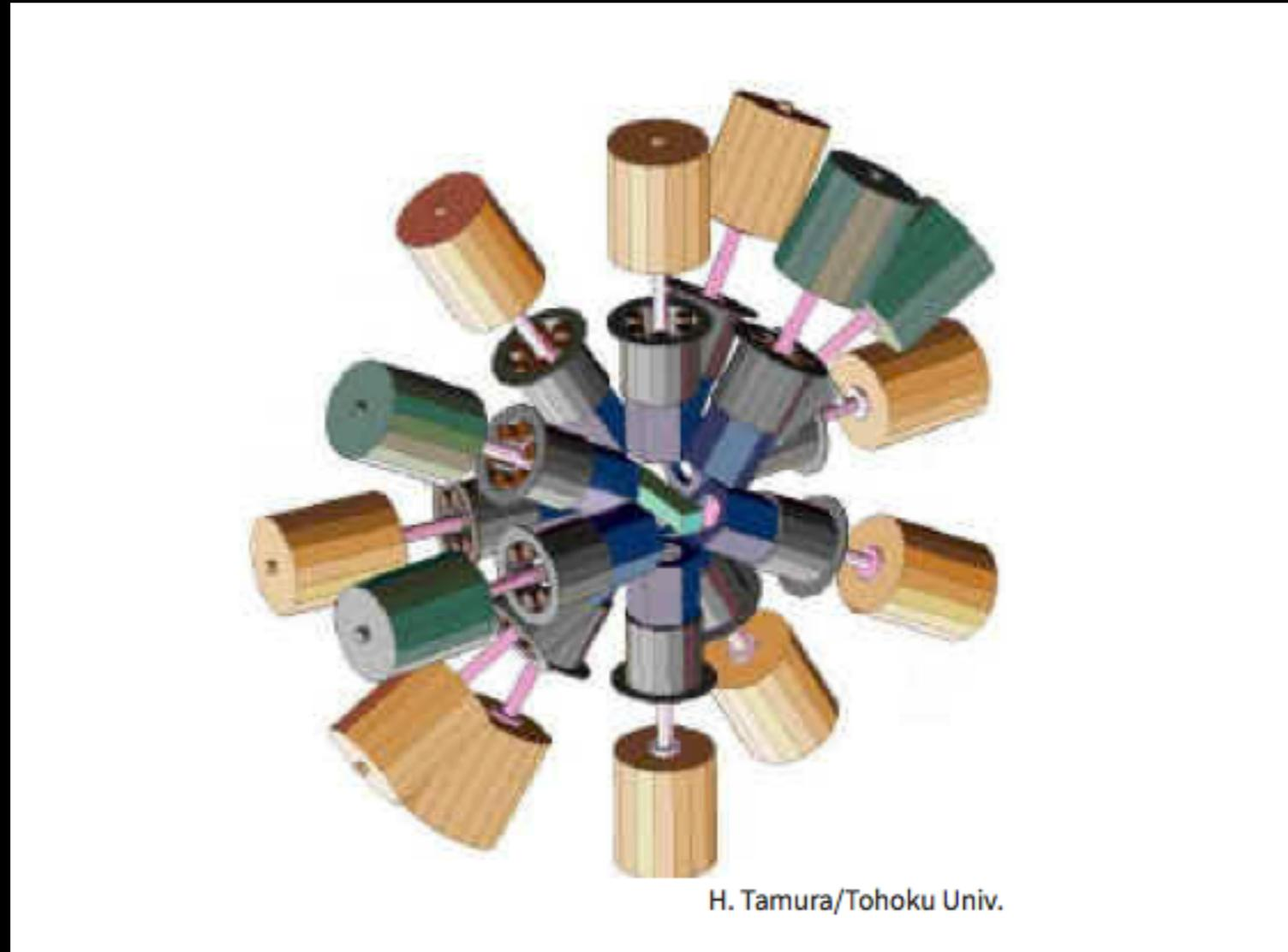
Hyperball consists of 14 high-resolution germanium detectors giving precision energy measurements of  $\gamma$ -rays
