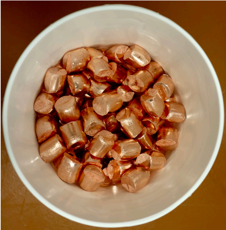
Copper nuggets before being placed in the electroforming baths. These have already been triple-etched in nitric acid.
