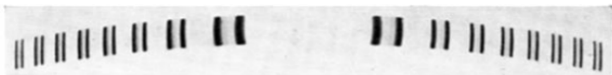
FIG. 3. Interferometer fringes of D\alpha obtained with a 5 mm étalon spacing.
